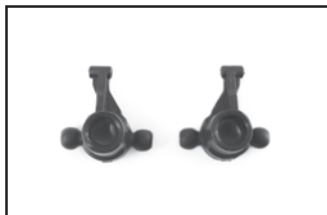
15410 4892793154109 GT248 FRONT HUB SET FRONT HUB L 1 FRONT HUB R 1
